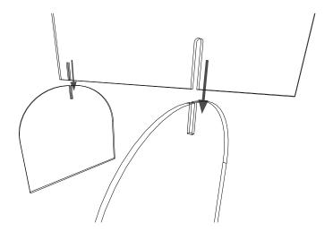
After removing protective coating, insert 2x legs into screen slots.
