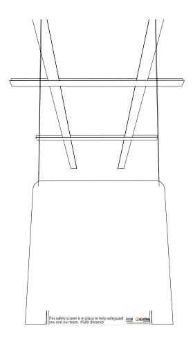
Suspend safety screen using fishing wire provided and adjust position to suit
